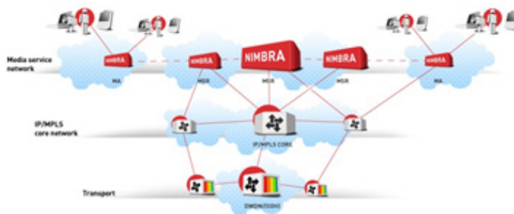
Equipment for video over fiber network
